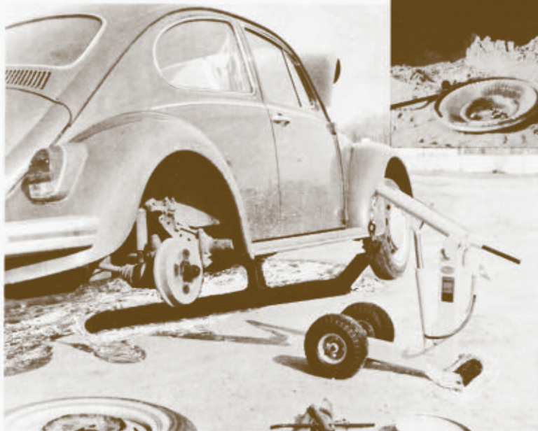
VEHICLE BEING LIFTED BY FRAME BAR AND JACK
